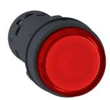
Monolithic illuminated push button, Harmony XB7, plastic, red, 22mm, integral LED, spring return, 230...240V AC, 1NO
