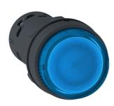
Monolithic illuminated push button, Harmony XB7, plastic, blue, 22mm, integral LED, spring return, 110...120V AC, 1NO
