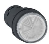
Monolithic illuminated push button, Harmony XB7, plastic, clear, 22mm, integral LED, spring return, 24V AC DC, 1NO
