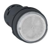
Monolithic illuminated push button, Harmony XB7, plastic, clear, 22mm, integral LED, spring return, 230...240V AC, 1NO
