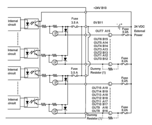
$<sup>^{(1)}</sup>$  (Example) The output delay time (OFF to ON) is 1.5  $\mu$ s where the output current is 50 mA. Install an external dummy resistor to increase the amount of current when faster response is required when the load is light.
