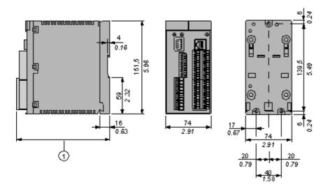
When using XPSMCTS+ connectors this dimension is 153 mm (6.02 in) When using XPSMCTC• connectors this dimension is 151,5 mm (5.96 in) Mounting and Clearance
