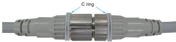
Note: Attach C-rings to both the plug and socket.
