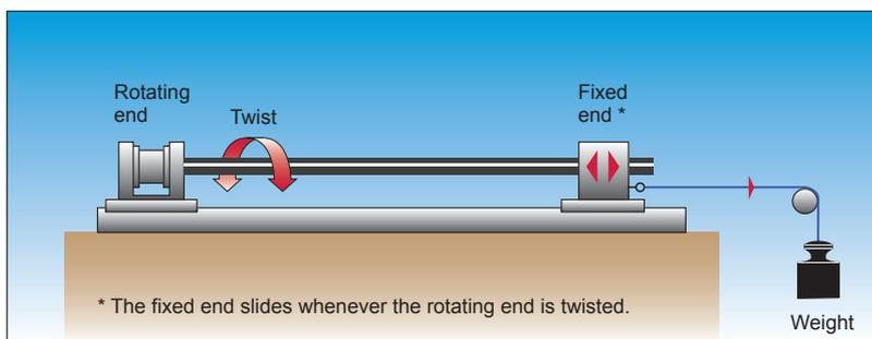
Torsion angle and length: PVC:  $\pm 180^\circ$  over 0.5 m
