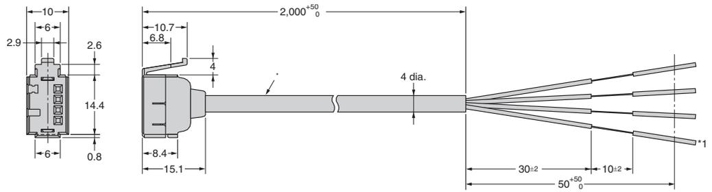
\* E3X-CN21: 4-dia. vinyl-insulated round cable with 4 conductors (Conductor cross section: 0.2 mm<sup>2</sup>, Insulator diameter: 1.1 mm)
