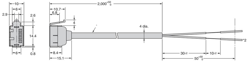
\* E3X-CN21: 4-dia. vinyl-insulated round cable with 4 conductors (Conductor cross section: 0.2 mm<sup>2</sup>, Insulator diameter: 1.1 mm)
