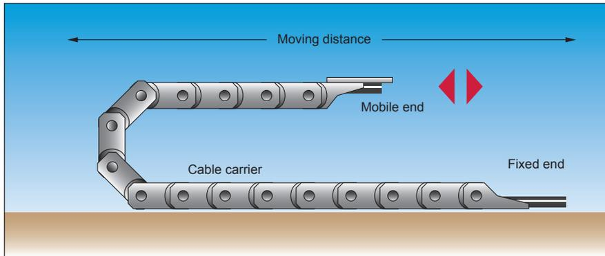
Cable carrier bending radius: approx.  $9 \times$  cable outer diameter
