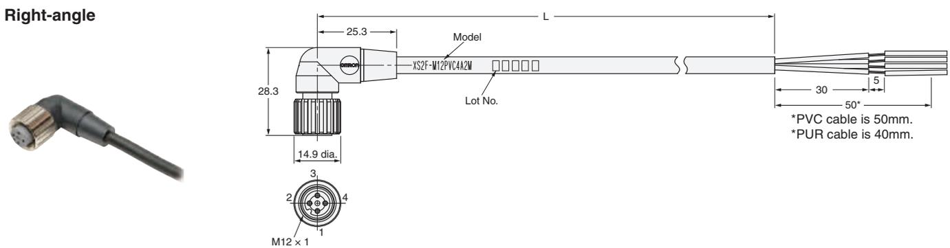
Note: For 3-core, pin 2 is not connected internally
