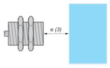
e (3) ≥ 45 mm/1.77 in. Mounted in a metal support
