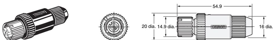
XS5C-D□S□ (Screw-on Connectors, Applicable Cable Outer Diameter: 3, 4, or 6mm)
