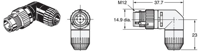
XS5G-D□S (Screw-on Connectors, Applicable Cable Outer Diameter: 7 or 8mm)
