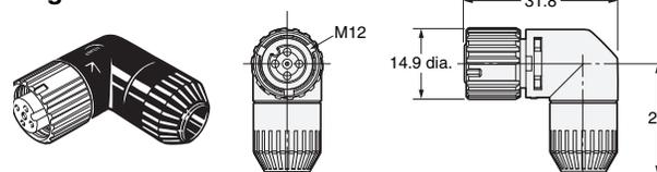
XS5C-D□S□ (Screw-on Connectors, Applicable Cable Outer Diameter: 7 or 8mm)
