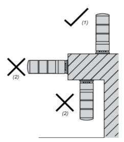
Choose a flat surface with enough strength and with little vibration for installation. Mount this product according to the figure to maintain IP characteristics
