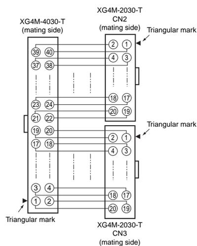
**MIL 20-pin - MIL 20-pin, Straight Wiring**
