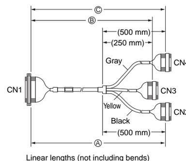
\*Up to two cables required for each Programmable Controller I/O Unit.
