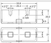
Note: The Cover has six thin, easy-to-separate portions for easy lead wire connections.
