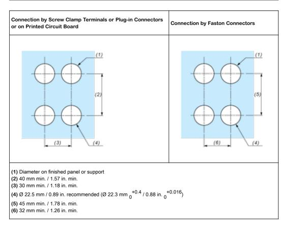
Pushbuttons, Switches and Pilot Lights for Printed Circuit Board Connection
