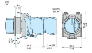
e : Clamping thickness : 1.2 to 2.8 mm / 0.05 to 0.11 in.(1) Additional row of contacts or double contact
