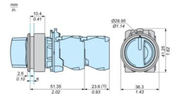
${\bf e}$  : Clamping thickness : 1 to 3.5 mm / 0.04 to 0.14 in. (1) Additional row of contacts or double contact
