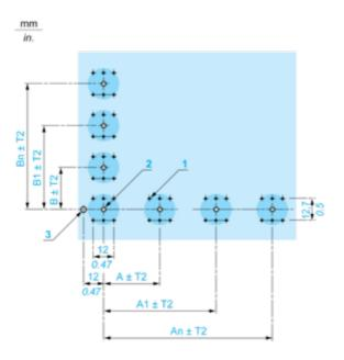
A 24 mm/0.94 in. minimum for rectangular heads, 18 mm/0.71 in. minimum for square or circular heads B 18 mm/0.71 in. minimum
