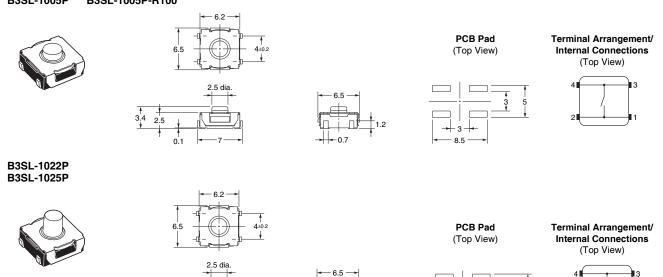
Note: Unless otherwise specified, a tolerance of ±0.4 mm applies to all dimensions. No terminal numbers are indicated on the Switches.
