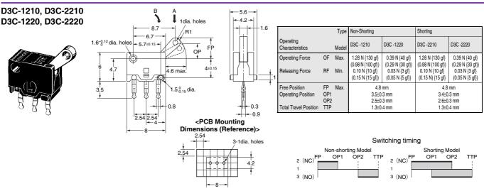
Note 1. Unless otherwise specified, a tolerance of  $\pm 0.4$  mm applies to all dimensions.
