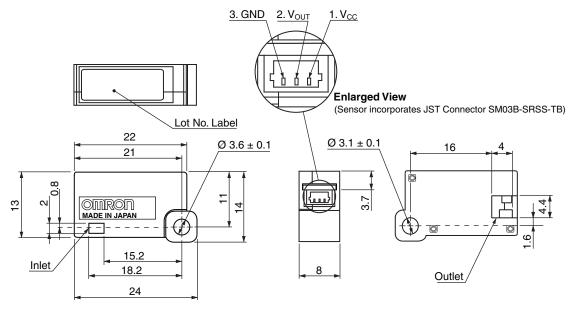
Note: Mount using M3 panhead screws, tightened to 0.59 N•m max. torque
