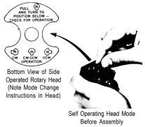
**Side Rotary -** The operating mode (CW, CCW or CW and CCW) of these spring return operating heads is easily changed without tools as shown in the illustration above. Remove the head from the switch body. Pull out the plunger and turn until its position matches that shown on the diagram for the desired operation mode. Levers are adjustable to any angle (360 degrees). The operating shaft screwriver slot can be used to maintain shaft position during lever installation.
