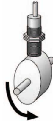
Eccentricity or Absolute Angle Detection
