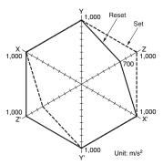
Sample: G6BK-1114P-US Number of Relays: 12 pcs Test Conditions: The value at which malfunction occurred was measured after applying shock to the Shock direction
