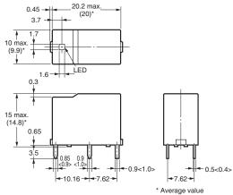
Dimensions in pointed brackets < > are for the Relay mounted to Socket.
